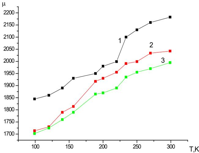
**Graph 19.** Dependence of magnetic permeability on temperature for composite with 50% Fe<sub>2</sub>O<sub>3</sub> + 50% BT at 3000 rpm, 1- H=602 A/m, 2- H=1200 A/m, 3- H=1800 A/m
