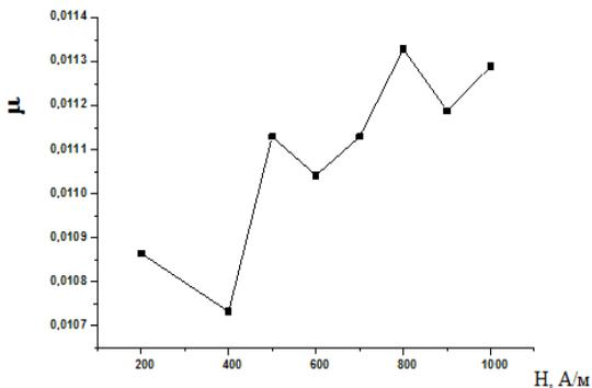
**Graph 23.** The dependence of the magnetic permeability on the value of the magnetic field for the composite with 50% Fe<sub>2</sub>O<sub>3</sub> + 50% BT(d<63μm).
