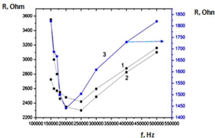
**Graph 13.** Dependence of the resistance on the frequency of the oscillating field: 1 – non-modified bentonite, 2 – modified bentonite at 3000 rpm – №.1, 3 – modified bentonite at 6000 rp/m – №.2 ( $U=1.14V$ )
