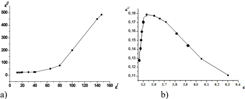
**Graph 3.** Cole-Cole diagram for composites a) 70% BT + 30% PE
