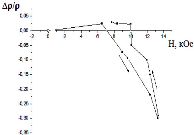
**Graph 22.** The dependence of the magnetoresistance on the value of the magnetic field for the composite with 50%Fe<sub>2</sub>O<sub>3</sub>+50% MBT.
