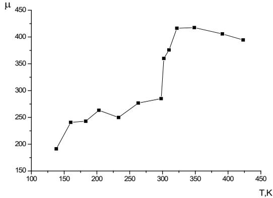
**Graph 20.** The dependence of the magnetic permeability on the temperature for the composite with 60%  $\text{Fe}_2\text{O}_3$  + 40% BT at 6000 rpm.  $H=602$  A/m,  $f= 200\text{Hz}$ .
