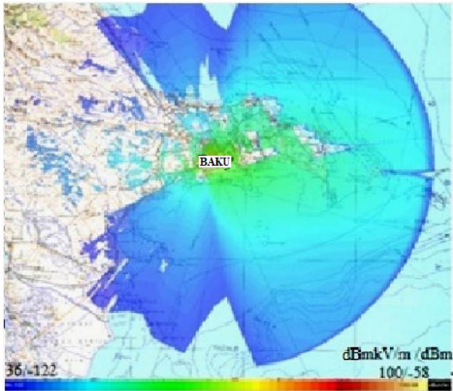
**Fig.3. Service area of the main radio transmitter**
