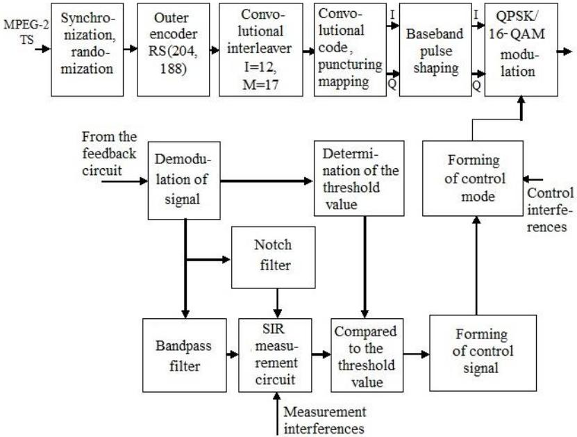
**Figure 1. Structural scheme of adaptive management of the modulation method on the down line of the LMDS system**
