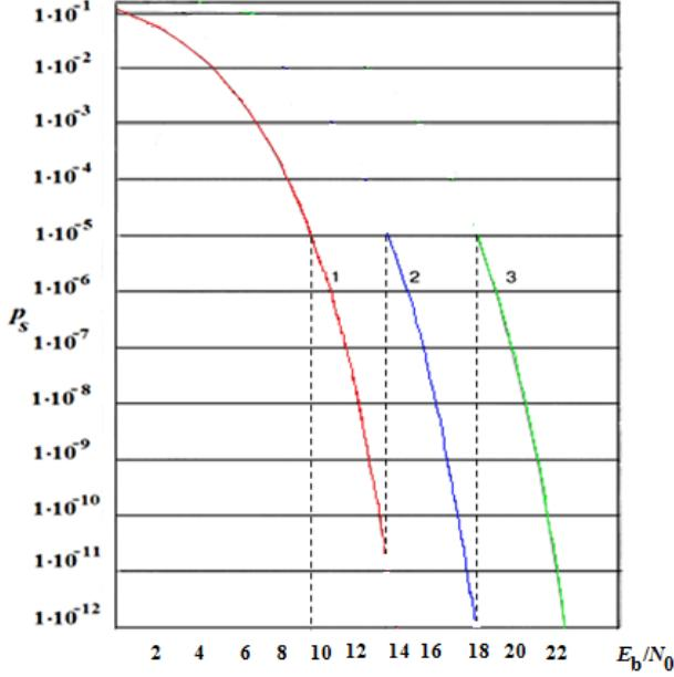
**Figure 2. Dependence of the error probability on the ratio  $E_b/N_0$  when changing the modulation method**
