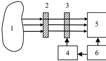
Fig.6. Flow chart of the narrow- band control system of objects on reflection spectrum: 1 - object, 2 – interference filter, 3 – controlled filter with liquid crystal, 4 – filter's control unit, 5 – acceptance and operation unit, 6 – control unit
