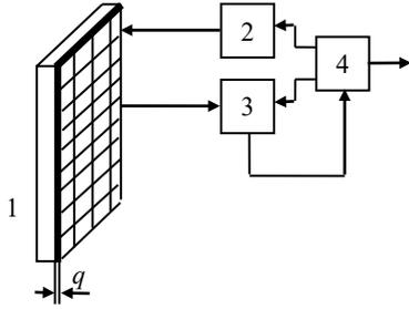
Figure.7. Flow diagram of X-ray fluorescence spectroscopic system: 1 a sheet with removed metal plate, 2 scanner type X-ray generators, 3-fluorescent signal photometric measuring device, 4 controlling calculator
