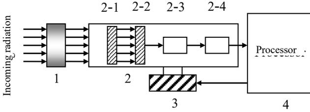
Figure.4. Functional diagram of differential spectrometer: 1- the substance under investigation, 2-spectrometer, 2-1-interference filter, 2-2-limiter, 2- 3-photo amplifier, 2-4-amplifier, 3-spectrometry orientation and rotation device, 4- processor
