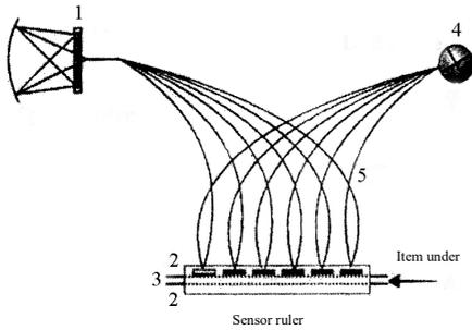
Figure.3. Technical realization reflexometric- interferometric spectroscopy principle: 1- spectrometer, 2- optical layer under mutual influence, 3-sensitive polymer layer, 4-light source, 5- light conducting fibers
