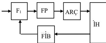
Figure 5. Functional scheme of adaptive photometric system:  $F_1$  -controlled narrow stripped interference filter,  $FP_2$  - photo- receiver, FIB -filter control block, ARÇ -analog-digital converter, İHG-controlling-computing device
