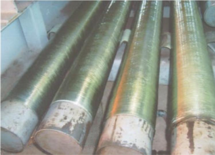
**Figure 2. General view of steel pipes insulated with composite plastic cladding on the outer surface**
